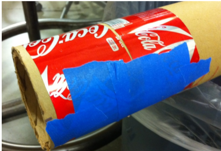
Figure 5.11. Close up of aluminum can surface on CFP. Blue tape is keeping tension on aluminum while the glue dries.
