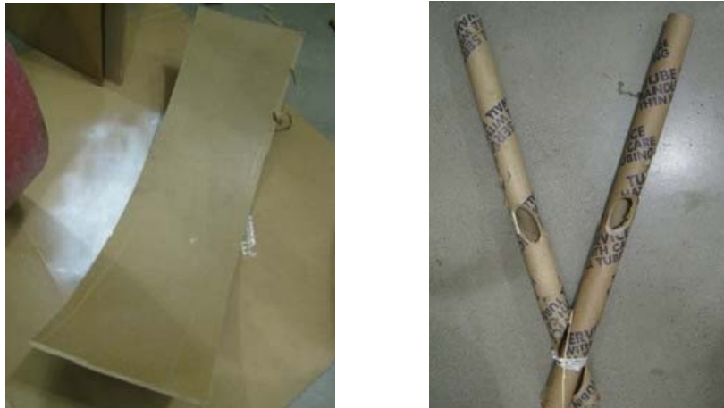
Figure 5.1. Curved Cardboard Platform and V-shaped Tube Supports
