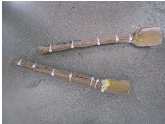
Figure 5.18. The components of the flag launching system. The figure on the left shows the loading spoons, which were reinforced with glue. The figure on the right shows the process of using the loading spoons to shove the flag inside the football.
