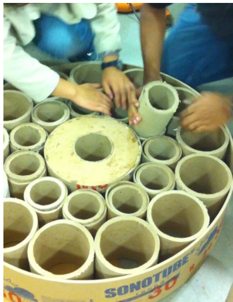
Figure 5.10. Concentric Tube Wheel construction—shimming the gaps between internal tubes.
