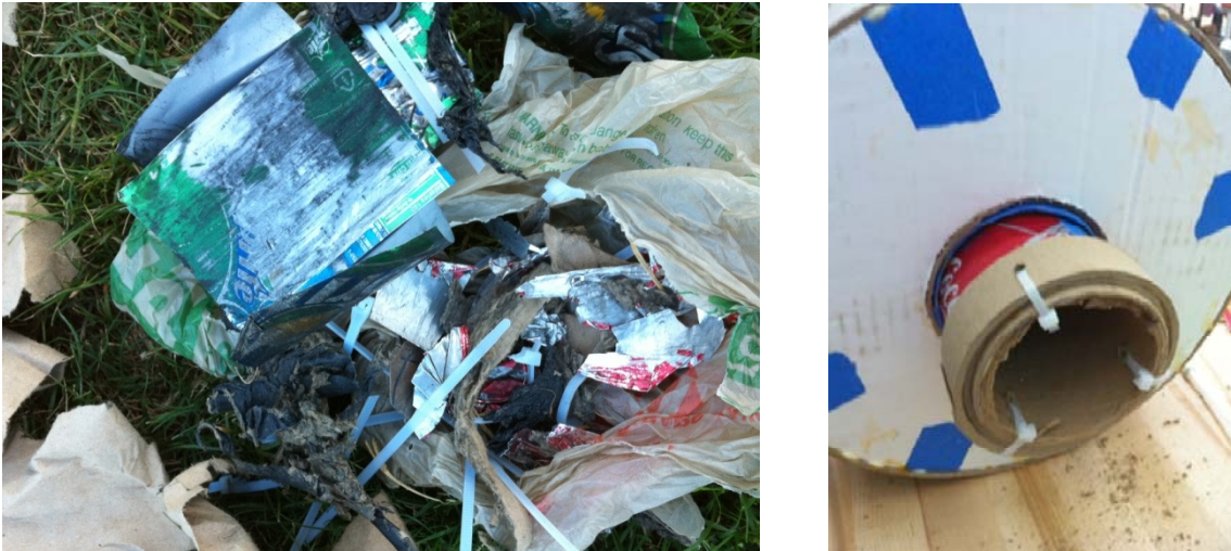
Figure 5.12. Photo (left) showing shrapnel from aluminum cans and shredded cardboard pulled from axle during break in PB Local Rally and additional photo (right) showing removable hub-cap design (zip ties), which allowed for quick serviceability during game play.
